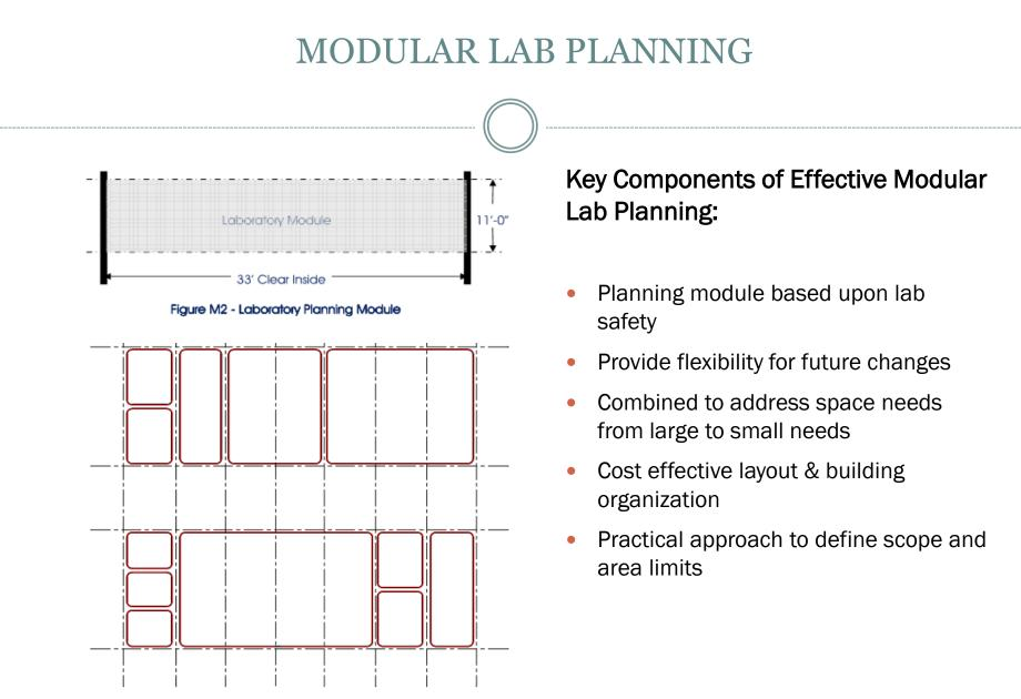
Figure M1 - Modular Planning of Laboratory Space
